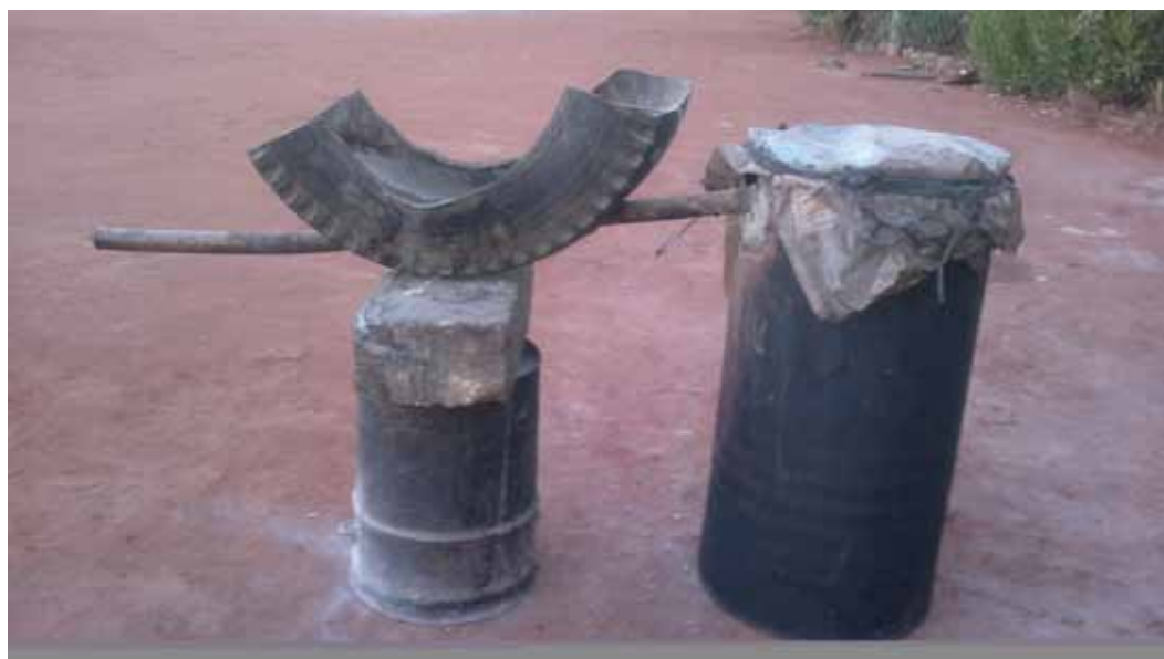
A still for producing sekhokho, or Bobirwa gin.
