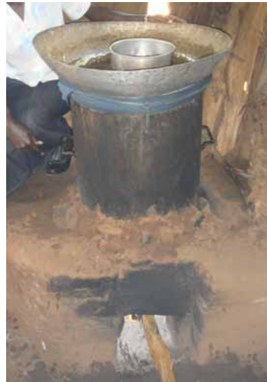
Complete setup of the distillation process for changaa production.
